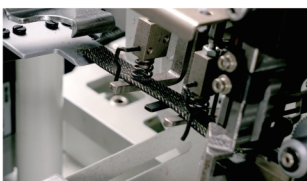
通过调整在斜切和直切模式之间转换 The conversion of chamfering and straight cutting modes
