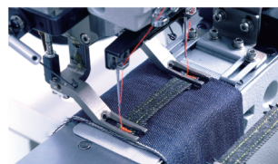
缝制时间提速到1.2秒 / 裤襻 (28针) Sewing time is accelerated to 1.2 seconds/belt loop (28 stitches)
